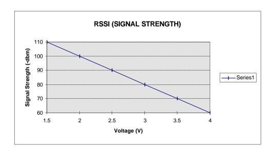
NOTE: The RSSI can be read remotely from the master radio if the SCADALink 900-MB is in Modbus mode.
