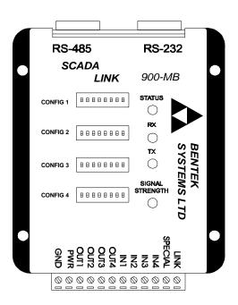
The following sections describe how to set up the DIP switches in each of 4 switch banks (config 1 - config 4). All 4 switch banks comprise of 8 bits labeled bit 1 to 8, starting from the left hand side of the switch bank.
